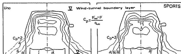
Fig. 21 - Pattern of total-pressure loss in the wake (looking down-stream)
