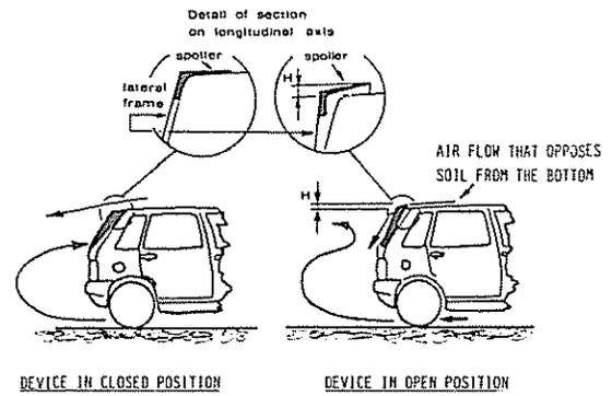
Fig. 24 - Diagram of back-window anti-soiling device
