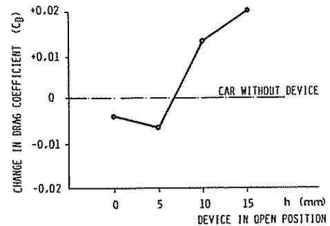
Fig. 25 - Influence of anti-soiling device on car drag
